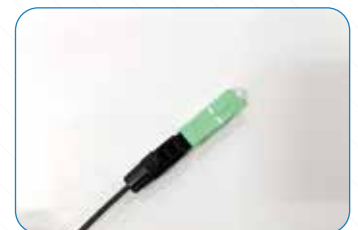
2.12 Lock the fiber (Take off the switch)
